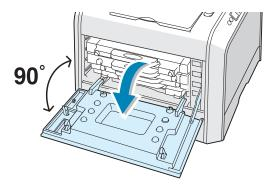
**3** Pull the handle lightly first, and then remove the used toner cartridge holding it.
